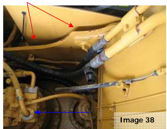
Image 38: Ensure that the small gap between the cabin wall and the base of the boom stick is cleaned and inspected. Contamination can often accumulate inside the small gaps where the hydraulic hoses connect, indicated here by the blue arrow.
