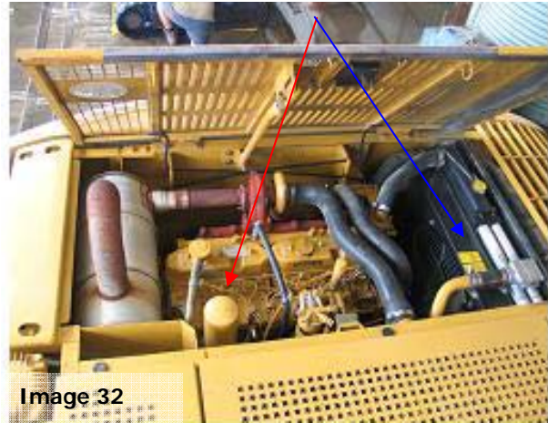
Image 32: The engine cover open, allowing access to the topside of the engine block (red) and radiator (blue).
