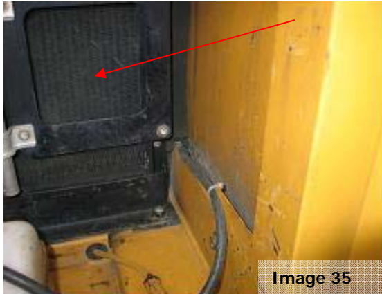
Image 35: On some models, a mesh grill protects the radiator core. These mesh grills need to be removed as the gauge is small and prevents contamination caught in the radiator fins from being successfully removed.
