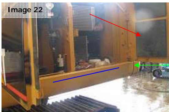
Image 22: A view of the LH side of the engine bay. Check all insulation foam (red arrow). The blue line again indicates that this section may be a hollow channel while the green line highlights the opening to this hollow section. This hollow section is not applicable on all models.
