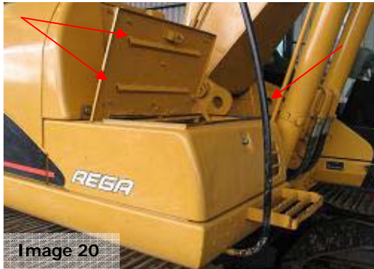
Image 20: The battery box located just in front of the fuel cell on the RH side of the excavator. Ensure the hollow, open-ended sections in the battery-box cover are flushed. Check handrail for openings at either end – flush if open-ended.
