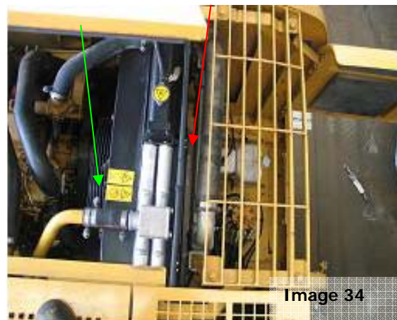
Image 34: The green arrow highlights the radiator shroud wire grill. This needs to be dismantled to allow access to the inside of the shroud and remove all contamination. The red arrow highlights the small gap between the radiator core and the oil-cooler cores. Check the cores by thorough flushing.
