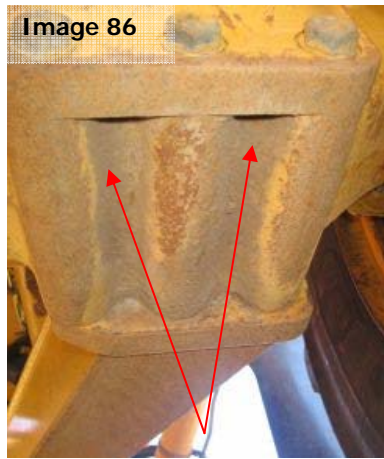
Image 86: The underside of the axel on the rear chassis. Ensure all contamination has been removed from this undulating surface.
