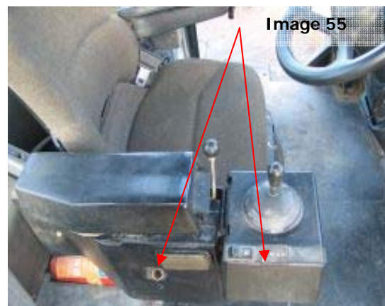
Image 55: Access will be required to the joystick control panels to verify internal cleanliness.
