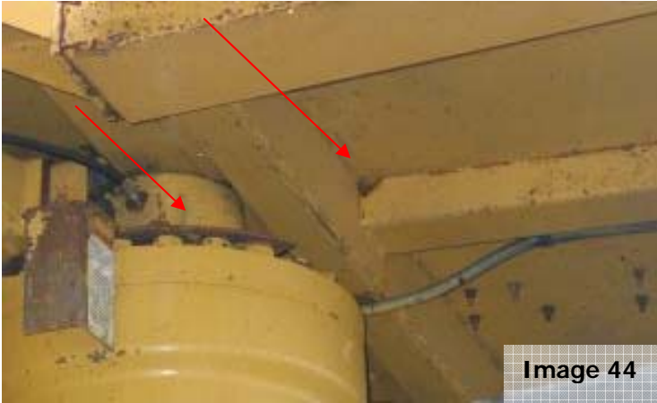
Image 44: Arrow indicates the small triangular openings that are found at the ends of these box sections.
