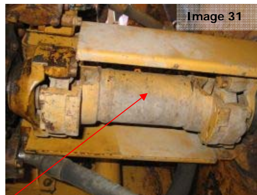
Images 30 & 31: The protective plate around the universal joint under the floorpan must be removed to facilitate the cleaning and inspection process. The second illustration shows the bottom half of the protective cover removed, allowing access to the universal joint.
