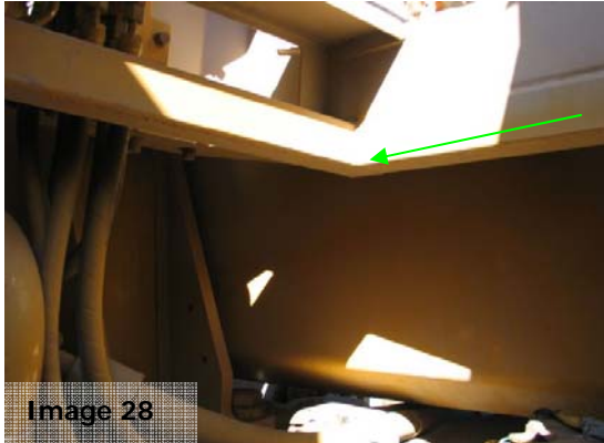
Image 28: Check all framework under the cabin floor. On some models this has open ends (green arrow), which will require flushing to verify cleanliness.
