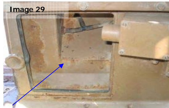
Image 29: The air-conditioning vent under the instrument panel has been removed for cleaning and inspection.
