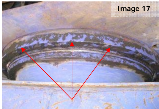
Image 17: All contaminated grease (red arrows) must be removed from the outer slew ring during the cleaning process.
