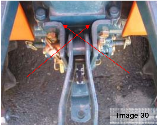
Image 30: Check for any contamination in areas where attachments are mounted to the rear of the tractor. Areas like those illustrated by the red arrows may require flushing to verify cleanliness.
