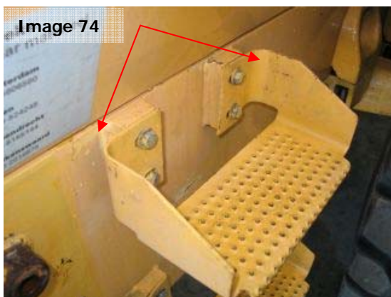
Image 75: The ladder to the cabin may have open-ended tubing (red arrows) that requires flushing to verify
