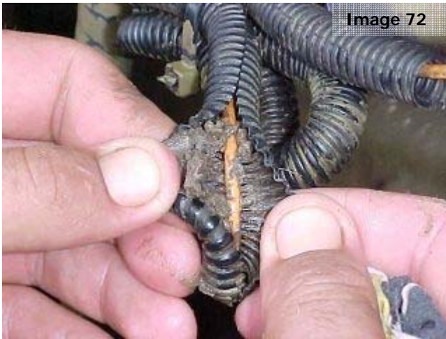
Image 73: Check all looming around hydraulic hoses for internal cleanliness.
