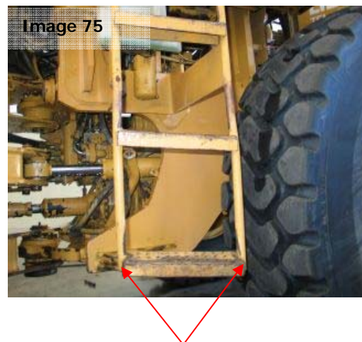
Image 75: The ladder to the cabin may have open-ended tubing (red arrows) that requires flushing to verify
